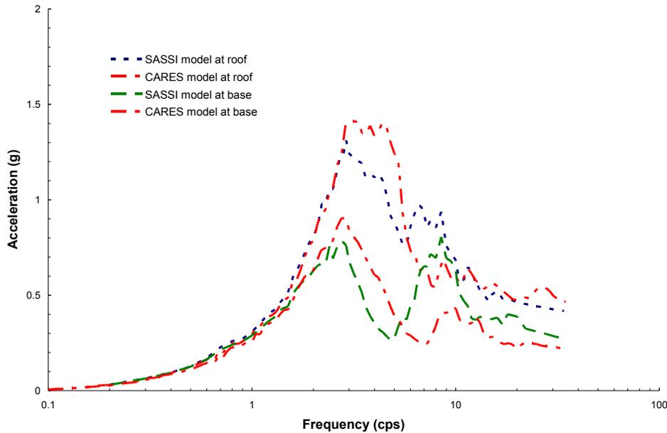
**Figure 8. Comparisons of SSI Response Spectra for 100% Embedment (E/R=3.40)**
