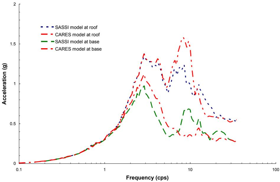
**Figure 7. Comparisons of SSI Response Spectra for 75% Embedment ( $E/R=2.55$ )**
