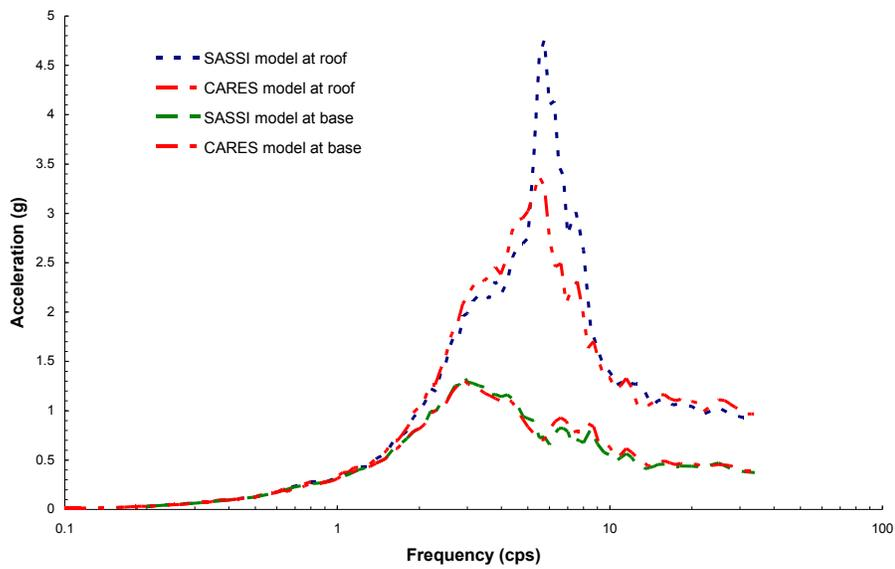
**Figure 5. Comparisons of SSI Response Spectra for 25% Embedment ( $E/R=0.85$ )**
