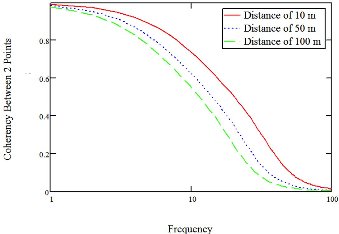
**Figure 9. Preliminary horizontal incoherency transfer proposed by EPRI**
