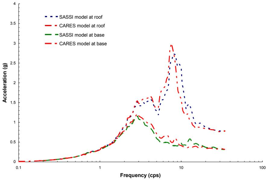
**Figure 6. Comparisons of SSI Response Spectra for 50% Embedment ( $E/R=1.70$ )**
